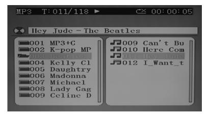
On the top line of the menu, "T: 011/118 means track #11 out of total 118 tracks is now playing. The elapsed time of current track is shown on the right.
